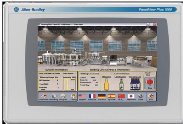
Figura 18. HMI Panel View plus 1000 - 10” – Allen Bradley.
